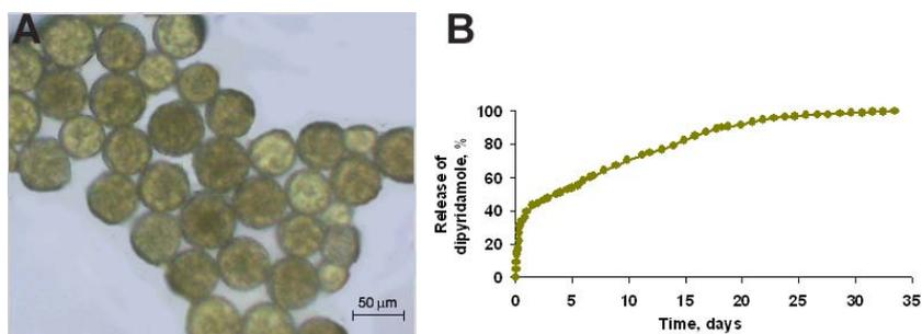
**Fig. 8.** PHB microspheres for sustained delivery of drugs. (A) PHB microspheres (average diameter = 60 μm, PHB Mw = 1000 kDa) loaded with dipyridamole (10% w/w); (B) Sustained delivery of dipyridamole from PHB microspheres for more than 1 month.
