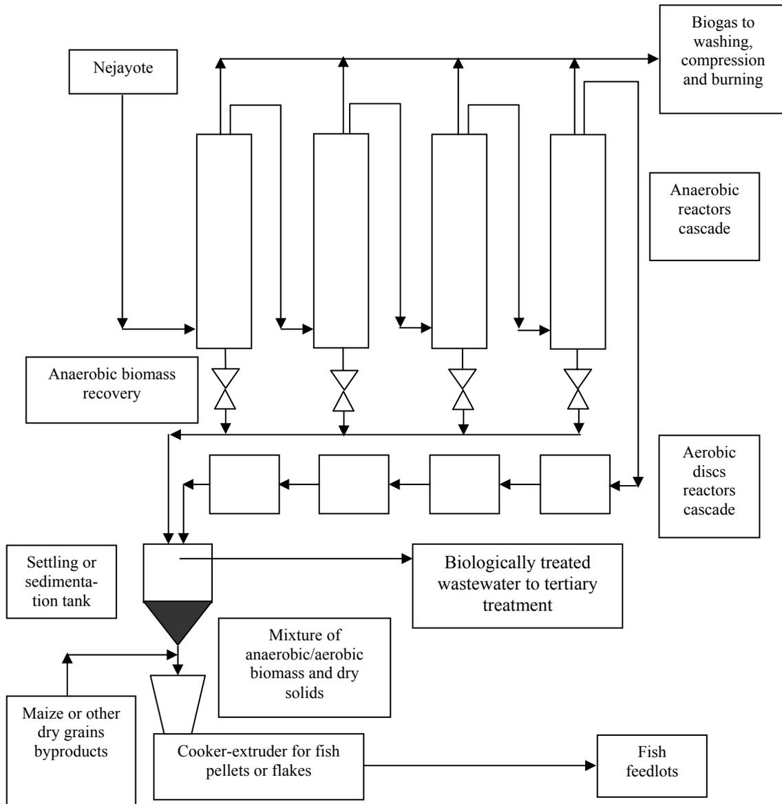
**Fig. 5** Block and flow diagram for the cornmeal factories wastewaters recycling [7].
