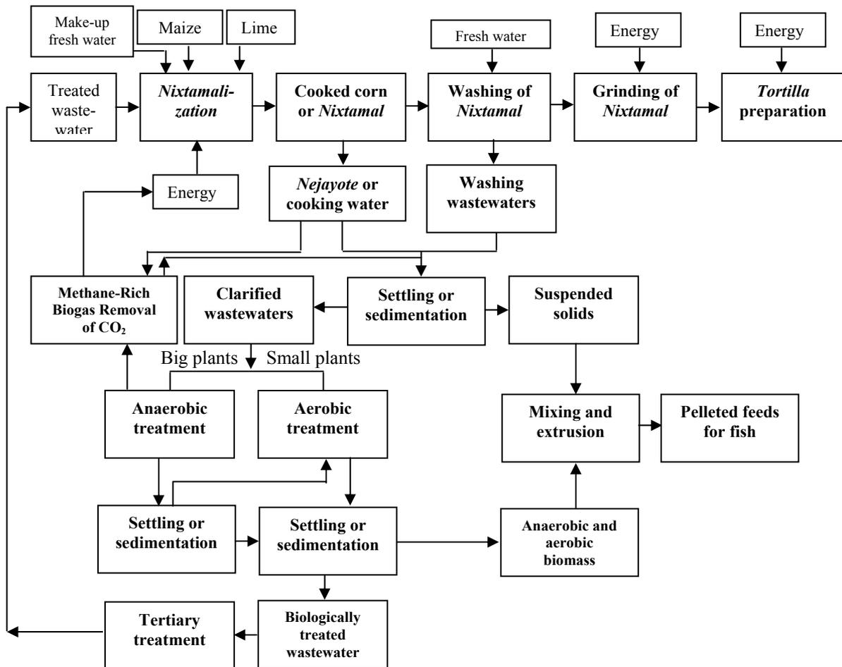
**Fig. 3** Proposed process to recycle maize processing wastewaters using anaerobic-aerobic treatment for big nixtamalized cornmeal factories and aerobic treatment for small corn dough plants.
