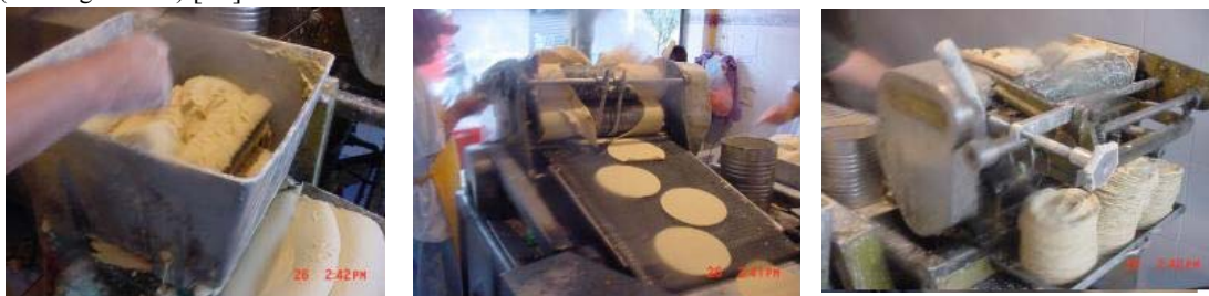
Fig. 1b Tortilla machine to form and cook alkaline prepared maize dough [3].
