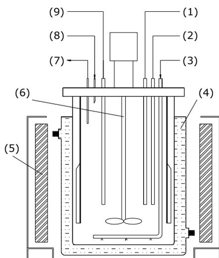
**Fig. 1** Scheme of the air-fluidized bed photobioreactor used in the experiments. The photobioreactor components are: (1) O<sub>2</sub> probe; (2) pH sensor; (3) Air and CO<sub>2</sub> supply; (4) Water jacket; (5) Light jacket; (6) Stirrer; (7) Medium outlet; (8) Medium inlet; (9) Temperature sensor.
