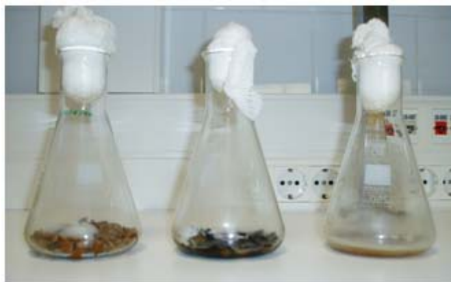
Fig. 1. Solid-state cultures of the white-rot fungus T. pubescens grown on different natural supports: mandarin peelings (left), banana skins (center) and wheat bran flakes (right)
