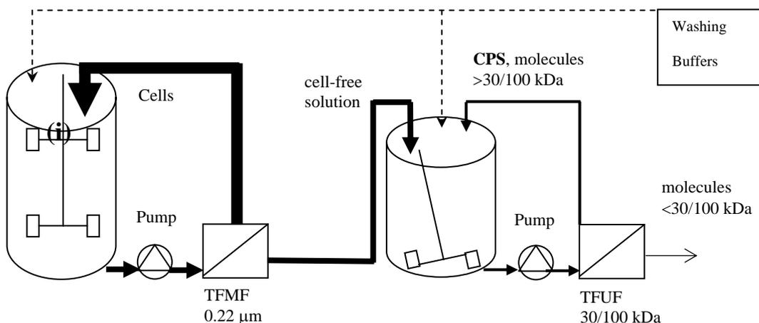
**Fig. 2** Scheme of cell separation by Tangential-Flow Microfiltration (TFMF) and concentration/diafiltration of cell-free microfiltrate and enzymatic treatment by Tangential-Flow Ultrafiltration (TFUF).
