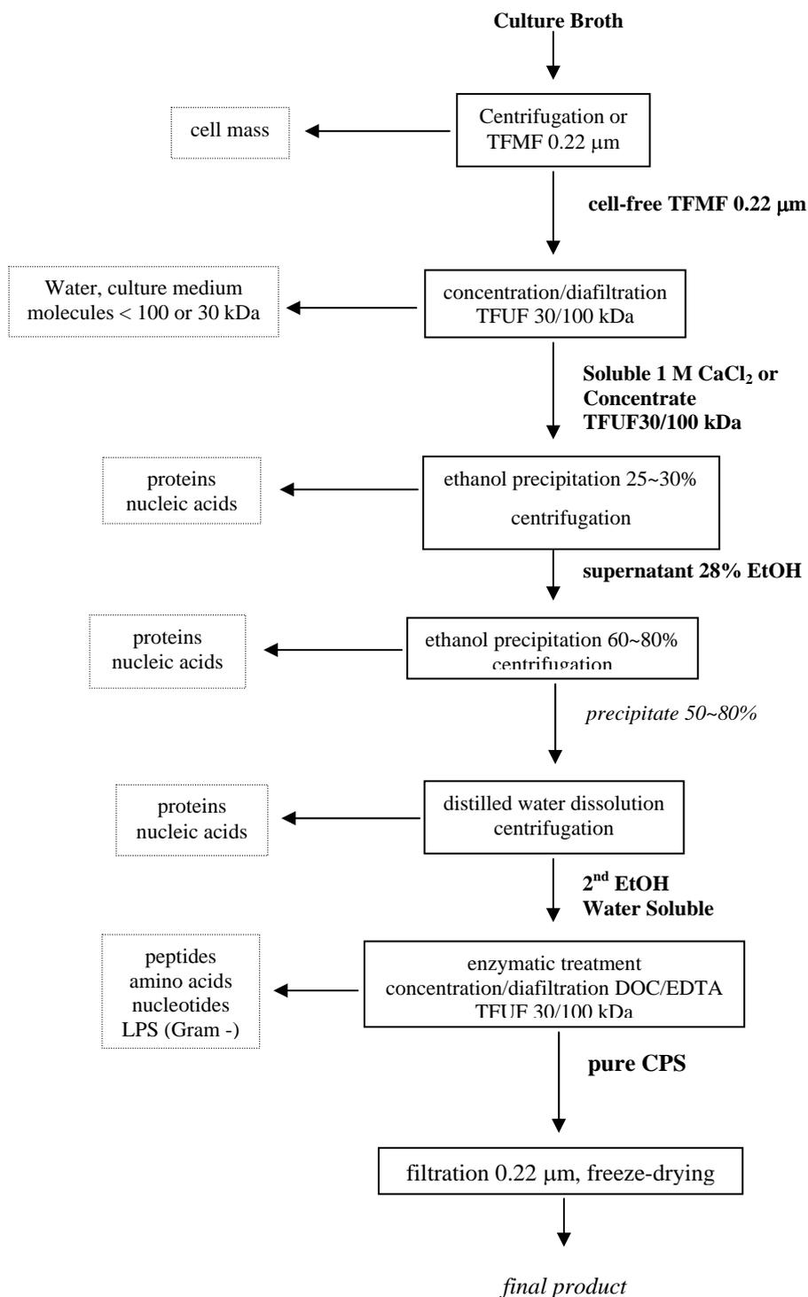
**Fig. 3** - Flow diagram of CPS purification process. Unit operations are in solid rectangles, main contaminants are in dotted rectangles, intermediate fractions presented in tables are in bold and intermediate fractions not presented in tables are in italic.
