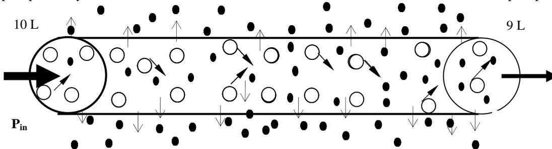
**Fig. 1** Scheme of Tangential Flow Microfiltration/Ultrafiltration.  $P_{in}$  = pressure inlet;  $P_{out}$  = pressure outlet. Transmembrane pressure -  $TMP = (P_{in} + P_{out})/2$
