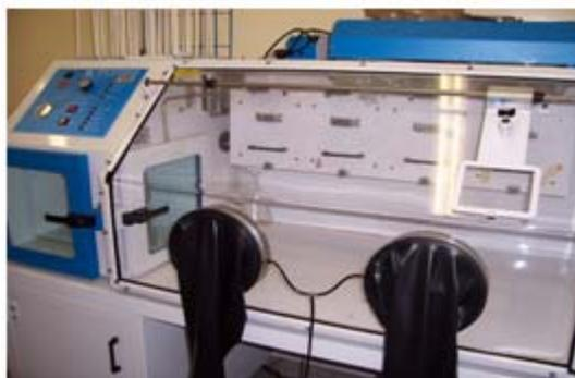
**Fig. 3** Bactron II anaerobic chamber.
