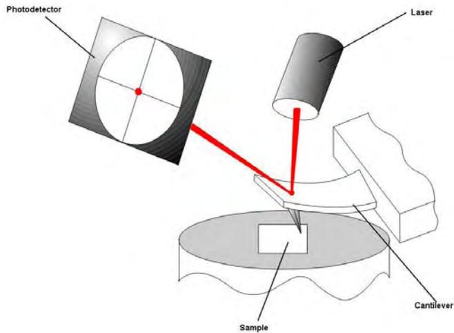
**Fig. 1** Schematic drawing of an AFM and of the sample positioned. An AFM consists of a flexible shaft with a tip at its extremity. The deflection signal is monitored by an optical system consisting of a diode laser and a photodetector that is sensitive to variations in position. Deflections of the sample are plotted point to point while scanning on surface.
