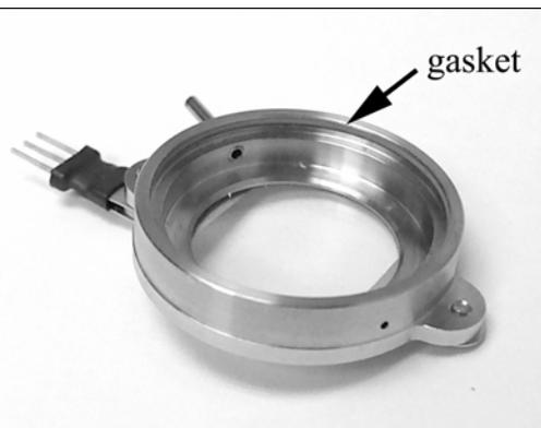
**Fig. 2** Biopetech dish with gasket installed.
