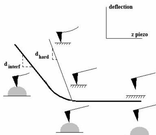
**Fig. 3.** Schematic drawing showing the AFM cantilever deflection as it approaches, touches and pushes a hard and a liquid surface. The extension of the contact part has been exaggerated; in a real experiment it should be kept as small as possible so that the interaction between the liquid surface and the AFM tip can be modeled as two linear springs in series, and also to avoid capillary wetting of the tip.
