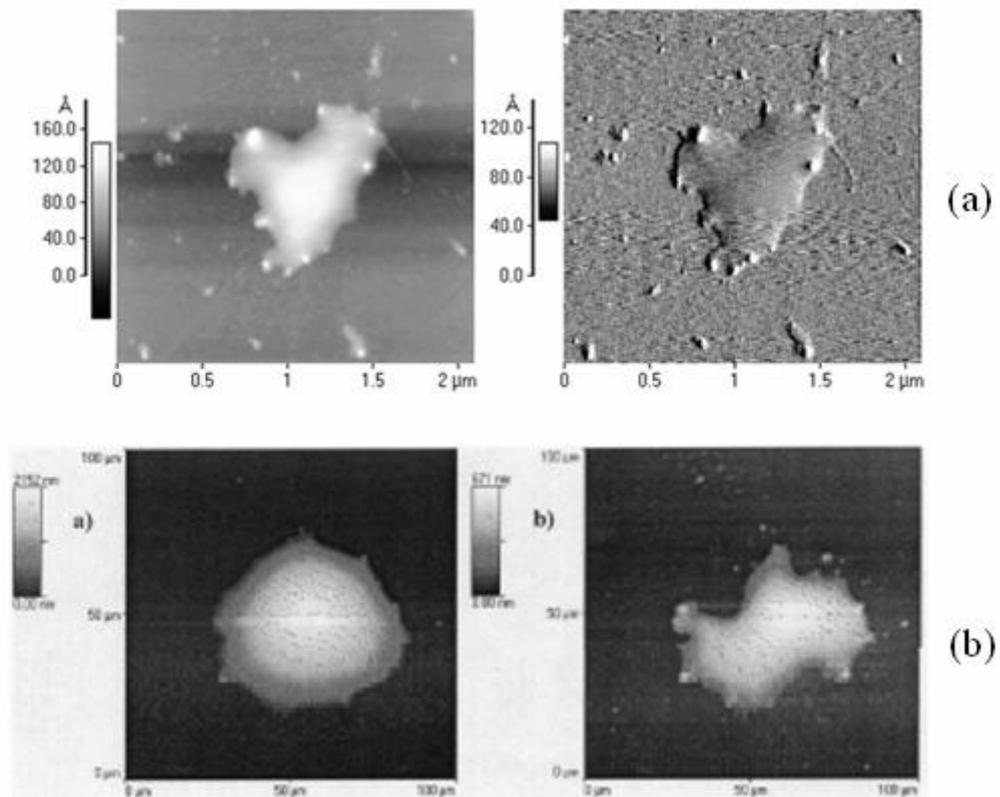
**Fig. 5. (a)** AFM images showing water micrometer-sized droplets-films, during the first stages of dewetting. (Left: topography; right: amplitude) [33]. **(b)** Dewetting sequence of a 1,5-pentandiol droplet right after deposition. The right image is taken 28 minutes after the left one. Note the similarity of both patterns (*a* and *b*-right), even at such different dimensional scales. Reproduced with permission from [34] © 2004 John Wiley & Sons.
