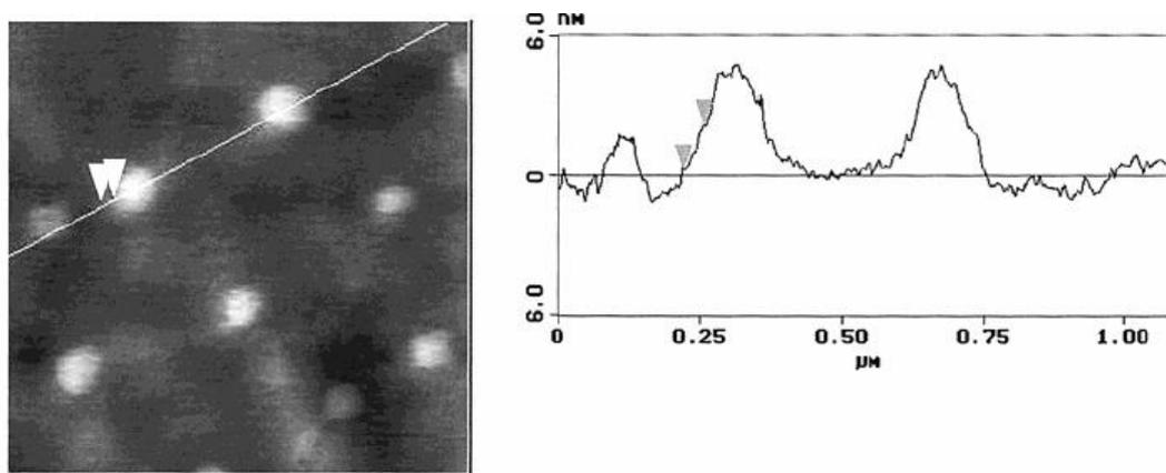
**Fig. 4:** Cross-sectional profile of oil droplets on a PS surface in water, taken in intermittent-contact AFM. Height of the droplets was about 5 nm and contact angle 4-5°. Reproduced with permission from [6]. ©2002 American Chemical Society.
