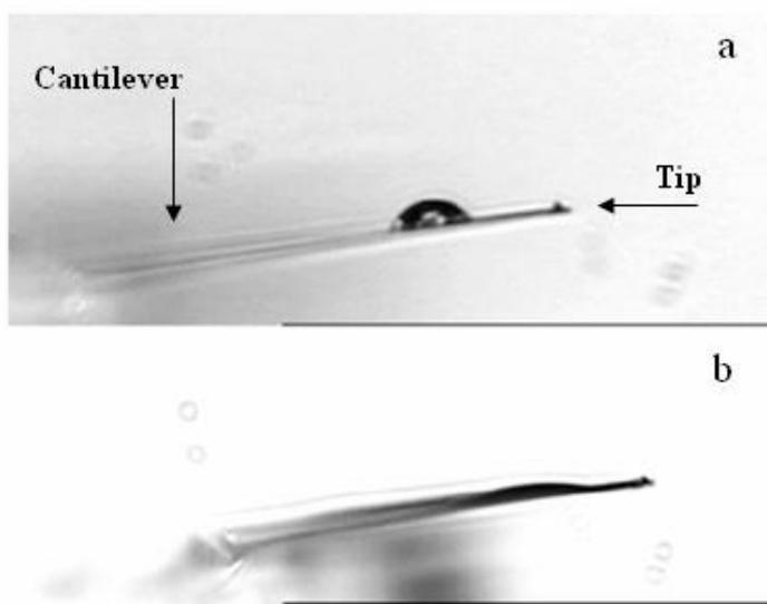
Fig. 2. Sequence of two images showing a water drop deposited on a V-shaped  $\text{Si}_4\text{N}_3$  cantilever before (a) and after (b) plasma cleaning. Reproduced with permission from [5]. © 2005 American Chemical Society.
