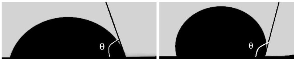
Fig. 1. Solid partly wetted by liquid (left); solid poorly wetted by liquid (right).
