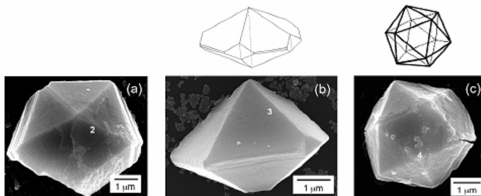
**Fig. 5** Superlattices of (a) pentagonal rod-like, (b) decahedral, and (c) icosahedral shapes. The sketches on the upper row show the geometrical model of Marks decahedron having re-entrant corners (for (b)) and that of icosahedron (for (c)) in the same orientations.
