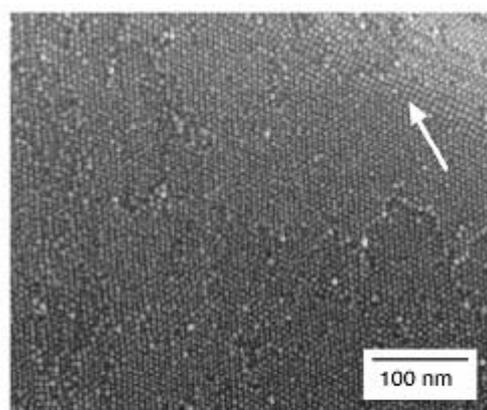
**Fig. 6** Magnified FE-SEM image at the vicinity of the edge region marked with 2 in Fig. 5a. The arrow indicates the truncated common edge.
