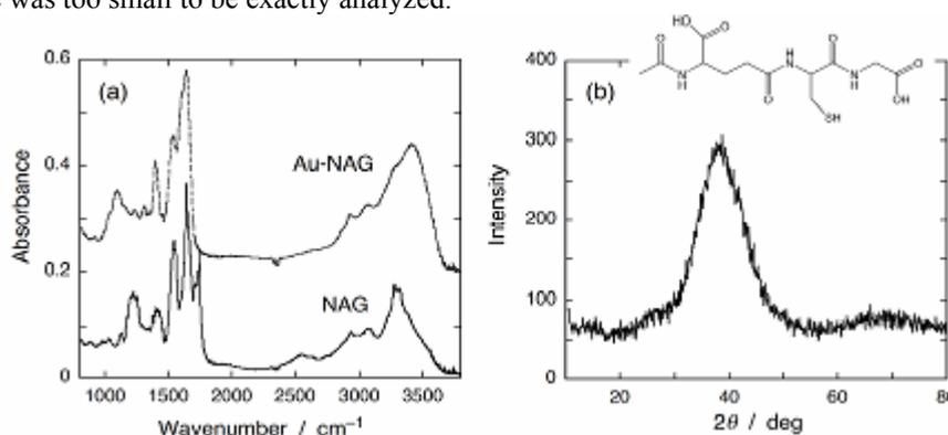
**Fig. 1** (a) FT-IR spectra of NAG and NAG-protected gold nanoparticles. (b) XRD profile of the as-prepared NAG-protected gold nanoparticles. The inset shows the chemical structure of NAG (*N*-acetylglutathione).
