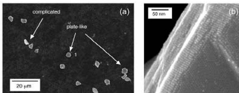
**Fig. 3** (a) FE-SEM image of the superlattices of NAG-protected gold nanoparticles on a Si substrate. The superlattices show a variety of morphology having well-defined facets. (b) Magnified image of the superlattice marked with 1.
