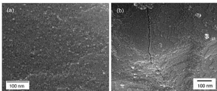
**Fig. 7** (a) Magnified surface image around the region marked with **3** in Fig. 5b. (b) Magnified surface image around the regions marked with **4** in Fig. 5c. The nanoparticle arrangement in the region of **3** differs from that of **2** or **4** of {111}-like planes.
