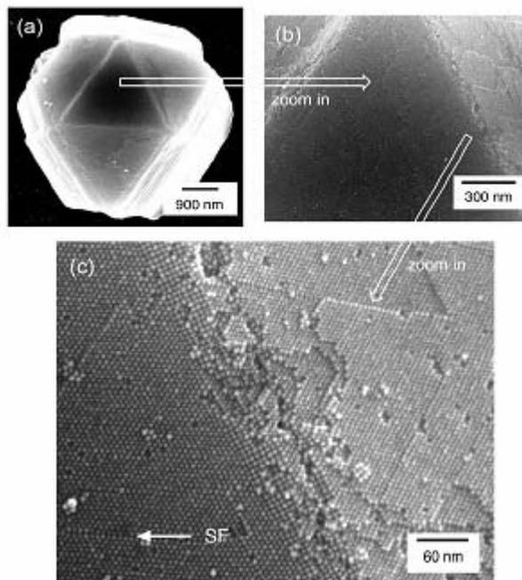
**Fig. 4** FE-SEM images of a superlattice of NAG-protected gold nanoparticles. (b) and (c) show the magnified surface images of the superlattice. The image in (c) clarifies the hexagonal close-packed arrangement of nanoparticles and a stacking fault. An example of the stacking fault is marked with “SF”.
