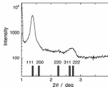
**Fig. 2** Small-angle XRD profile of the superlattice sample, suggesting a nanoscale periodicity caused by the formation of ordered arrays of gold nanoparticles.
