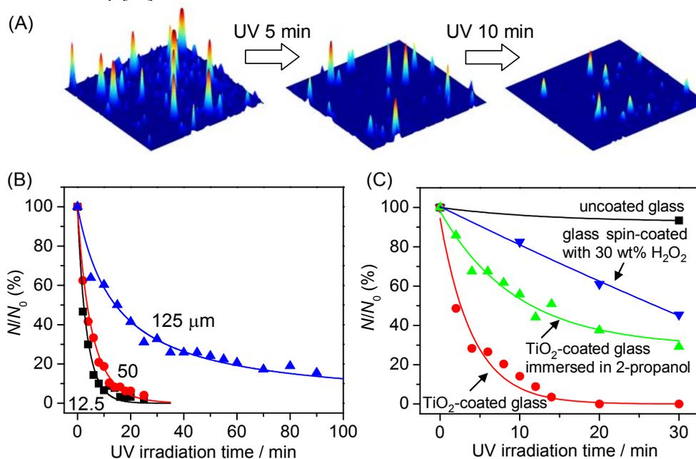
**Fig. 3** (A) Fluorescence images observed during the 532-nm excitation of single dye molecules immobilized on the coverslip before and after UV irradiation. (B) Time dependence of the  $N/N_0$  values in the gaps of 12.5, 50, and 125  $\mu\text{m}$ . The solid lines are visual guides. (C) Time dependences of the  $N/N_0$  values in the 12.5  $\mu\text{m}$  gap observed under various conditions. Copyright 2005 American Chemical Society.
