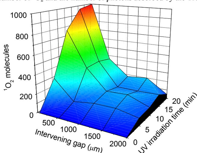
**Fig. 6** The spatial and temporal distributions of  $^1\text{O}_2$  molecules diffused from the surface of  $\text{TiO}_2$  film. The observation region is  $70 \times 70 \mu\text{m}^2$ . The intervening gaps are 50, 500, 1000, 1500, and 2000  $\mu\text{m}$ . Copyright 2006 American Chemical Society.
