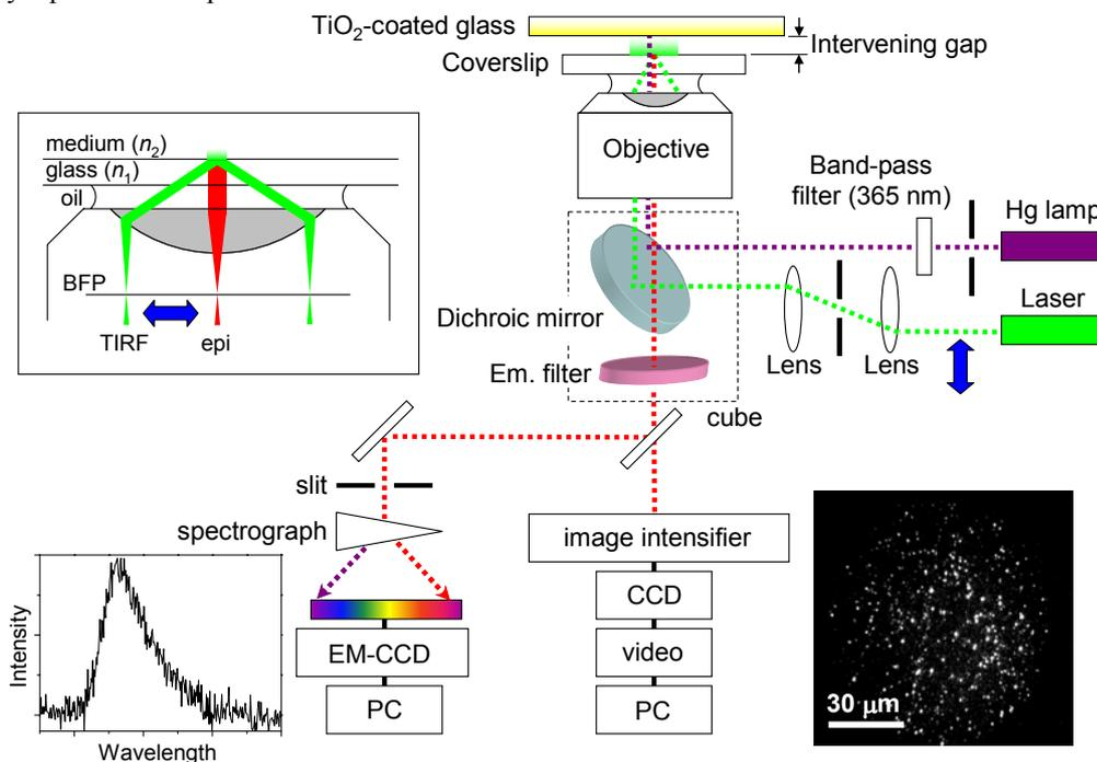
**Fig. 1** The optical configuration of objective-type TIRFM based on an inverted microscope.
