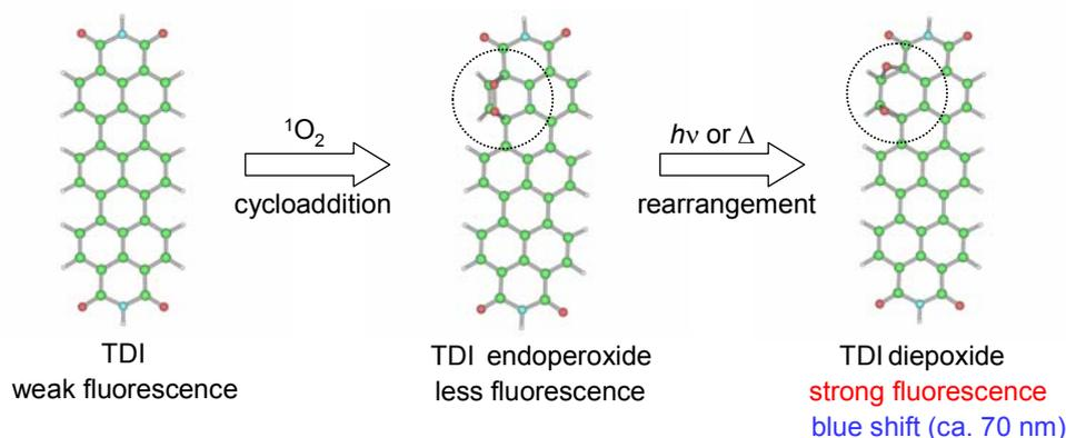
**Fig. 4** Single-molecule detection of  $^1\text{O}_2$  with TDI. Copyright 2006 American Chemical Society.
