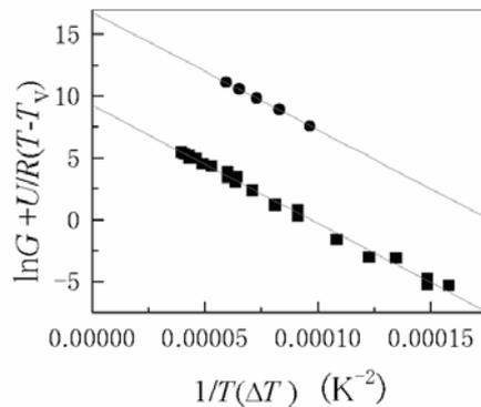
**Fig. 4** Plot of  $\ln G + U/R(T-T_v)$  versus  $1/T\Delta T$ . Symbols are the same as in Figure 3. The parameters used for the plots are as follows:  $T_m^0 = 128^\circ\text{C}$ ,  $T_v = -84.2^\circ\text{C}$ ,  $U/R = 758$  [1].
