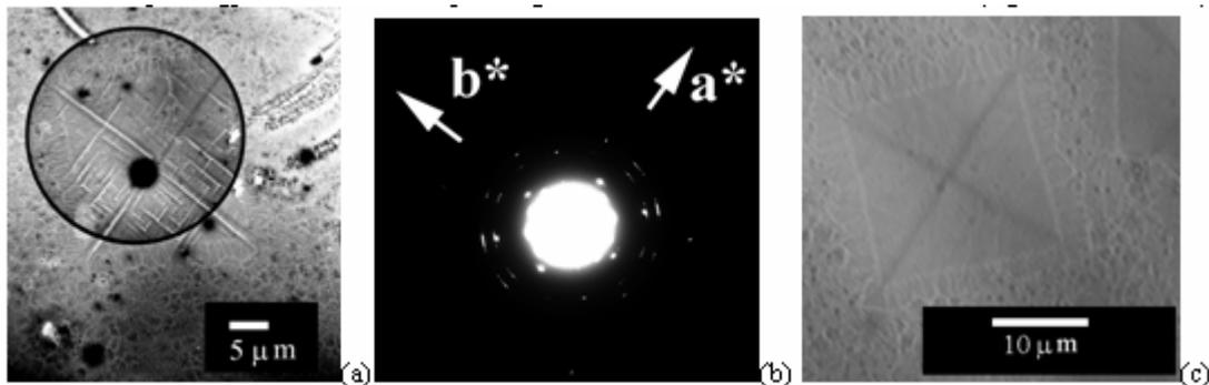
**Fig. 5** (a) Electron micrograph and (b) diffraction pattern of *it*-PB1 single crystal grown at  $100^\circ\text{C}$ . The solid circle in (a) shows the selected area for the diffraction. (c) Optical micrograph of an *it*-PB1 single crystal grown at  $100^\circ\text{C}$ .
