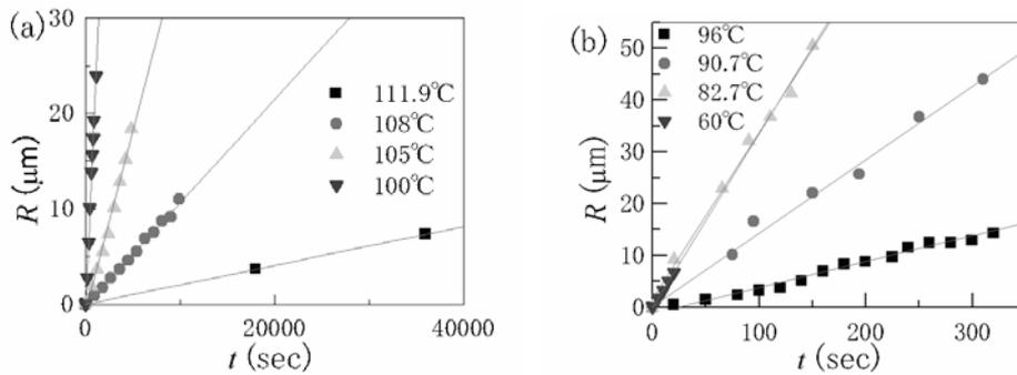
**Fig. 2** Time dependence of radius  $R$  for several crystallization temperatures. (a): (■) 111.9°C, (●) 108°C, (▲) 105°C, (▼) 100°C. (b): (■) 96°C, (●) 90.7°C, (▲) 82.7°C, (▼) 60°C.
