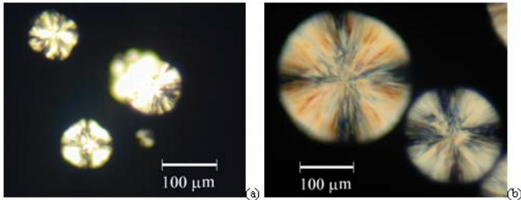
**Fig. 1** Optical micrographs of *i*-PB1 crystallized in the melt at 90°C; crossed polars. (a) 3 min and (b) 8 min after the temperature reached 90°C.
