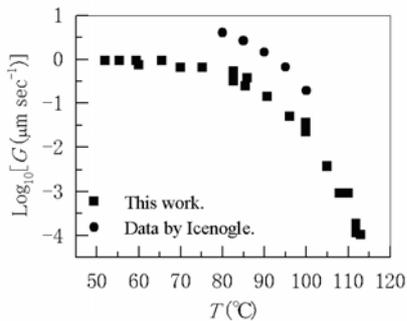
**Fig. 3** Growth rate  $G$  versus crystallization temperature  $T$ : (■) this work and (●) data by Icenogle [10].
