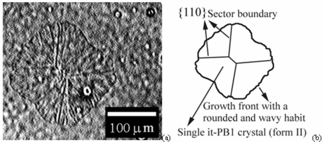
**Fig. 6** (a) *In-situ* optical micrograph and (b) schematic illustration of an *it*-PB1 single crystal growing at 85°C.
