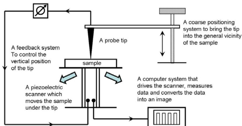
Fig. 1. Schematic of a generalized SPM.
