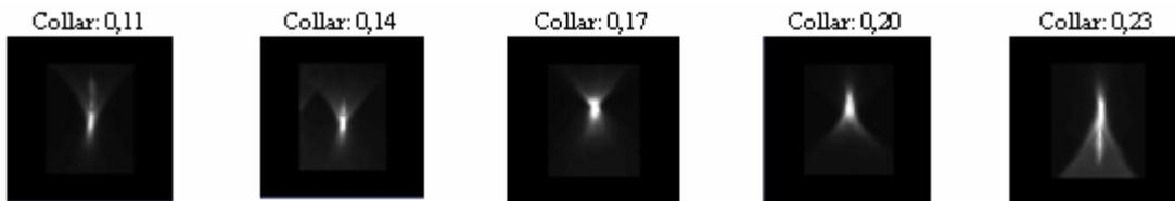
**Fig. 4B:** XZ projection of the PSF determined with a 40X 0.85 NA lens, using different correction collar values. In each case, conic figures with various degrees of asymmetry respect to the focal plane are observed.
