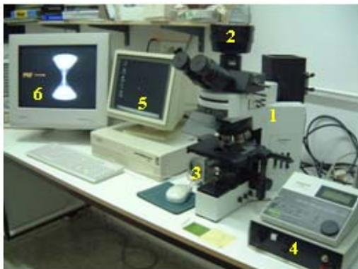
**Fig. 2:** DDM system designed and developed in the Microscopy Laboratory (FI-UNER), used to perform 3D studies.
