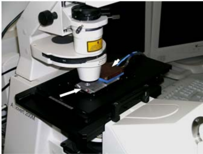
Fig. 2 Micrograph showing the arrangement of the specimen holder (arrow) and temperature generator (arrowhead) of the LM-TCC constructed by Buchner et al. [2] at a Zeiss Axiovert 200 M inverted Microscope. The temperature generator which includes the Peltier-Element is connected to the specimen holder on one side allowing proper illumination of the specimens in the specimen chamber
