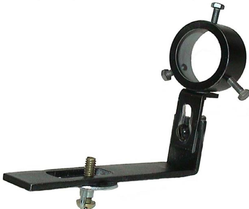
Figure 3. Photo of the camera microscope coupling device.
