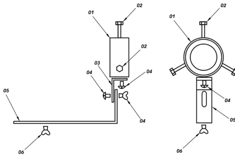
Figure 2. Diagram of the camera microscope coupling device.
